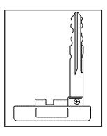
This key, located inside the keyless access transmitter, can be used for the driver's door, glove box, and rear seat pass-through door. See "Rear Seat Pass-Through Door" under *Trunk on page 2-20* for more information.
